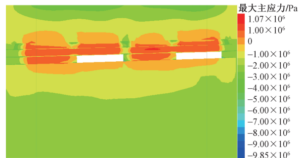
图 18 最大主应力云图(采场第三分层右侧) Fig. 18 Contour map of maximum principal stress (right side of the third layer of the mining site)
