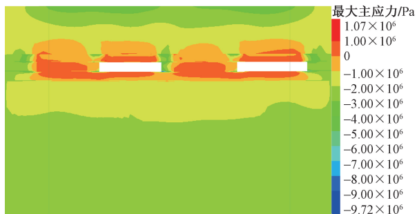
图 10 最大主应力云图(采场第二分层右侧) Fig. 10 Contour map of maximum principal stress (right side of the second layer of the mining site)
