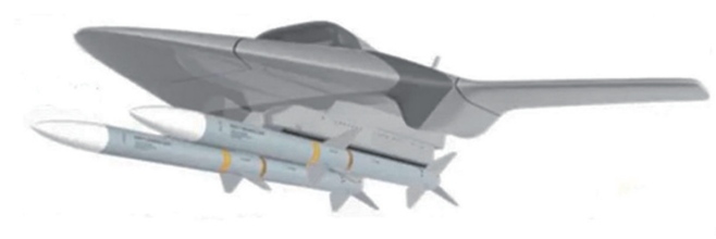
图4 飞行导弹导轨(FMR)示意 Fig.4 Concept of Flying Missile Rail
