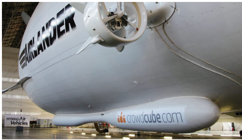
图31 AirLander 10管道状气垫着陆器 Fig. 31 Profiled pneumatic tubes ACLS of AirLander 10 airship
