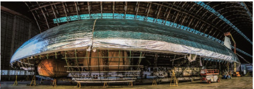
图22 Dragon Dream飞艇硬式蒙皮 Fig. 22 Rigid skin of Dragon Dream airship
