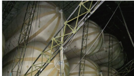
图20 Dragon Dream飞艇内部压力气囊 Fig. 20 Inner air bags of Dragon Dream airship
