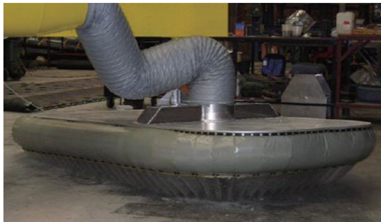
图34 P-791飞艇气垫着陆器模型及试验平台 Fig. 34 Model pad and test rig of P-791 airship ACLS
