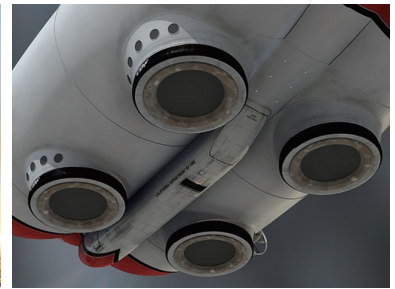
图33 P-791飞艇四点盘式气垫着陆器 Fig. 33 Four-point disklike ACLS of P-791 airship
