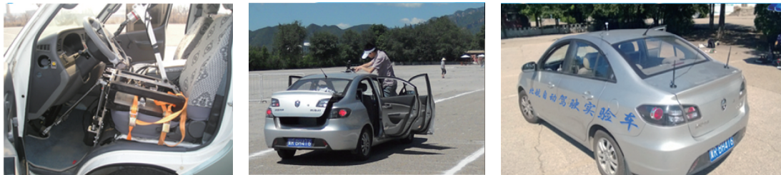
图10 Robot Driver型驾驶机器人安装和测试现场 Fig. 10 Installation and test site of Robot Driver
