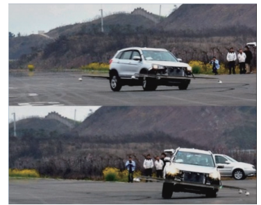
图6 汽车防侧翻试验 Fig. 6 Anti rollover test of vehicle
