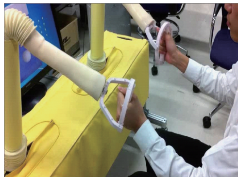
图 14 用于双手协调运动功能康复的机器人系统 Fig. 14 Development of a robot system for rehabilitation of upper limbs cooperative movement functions
