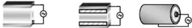
(a) 金属平板式 (b) 金属平板介质阻挡层式 (c) 同轴管状式 (a) Parallel plates (b) Parallel plate with bare electrodes dielectric-covered electrodes (c) Coaxial jet
