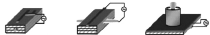
(a) 线性微波带式 (b) 基于微波带的表面波式 (c) 同轴管状波耦合式 (a) Microstrip (b) Microstrip linear resonator with engineered end (c) Coaxial jet linear resonator
