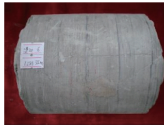
(e) 涩 20 井 (1281.4m), 浅湖环境, 浪成沙纹交错层理 (e) Well Se20 (1281.4m), shallow lake, wave ripple cross bedding
