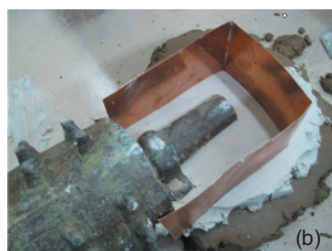
图 6 甬钟修复过程 2, (a)为分模线位置 Fig. 6 The second process of restoration, and figure (a) is the parting line
