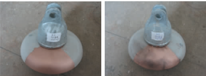
图 4 闪络前后绝缘子表面涂层状况 Fig. 4 Comparison of insulator surfaces before and after flashover
