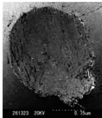
(a) 基础油中磨损后的钢球 (a) Frayed steel ball in fundamental oil
