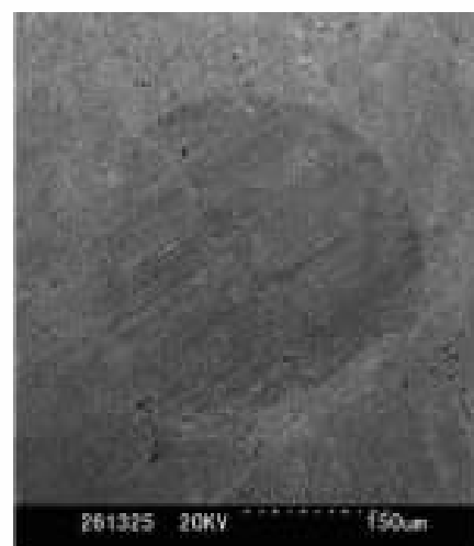
(b) 添加 PyDDP 后磨损后的钢球 (b) Frayed steel ball in the oil added PyDDP
