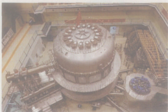
图2 EAST全超导托卡马克核聚变实验装置 Fig. 2 The experimental device of nuclear fusion, EAST (Superconducting Tokamak)
