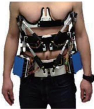
图10 用于脊柱畸形矫正的躯干外骨骼 RoSE Fig. 10 Robotic Spine Exoskeleton (RoSE) for human torso
