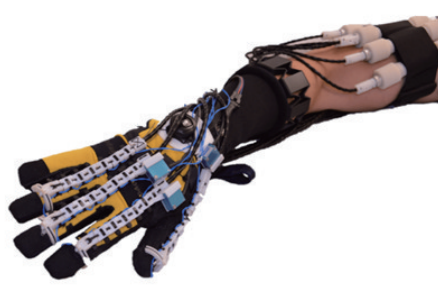
图8 刚柔混合型手外骨骼手套 SPAR Fig. 8 SPAR glove with rigid-soft exoskeleton
