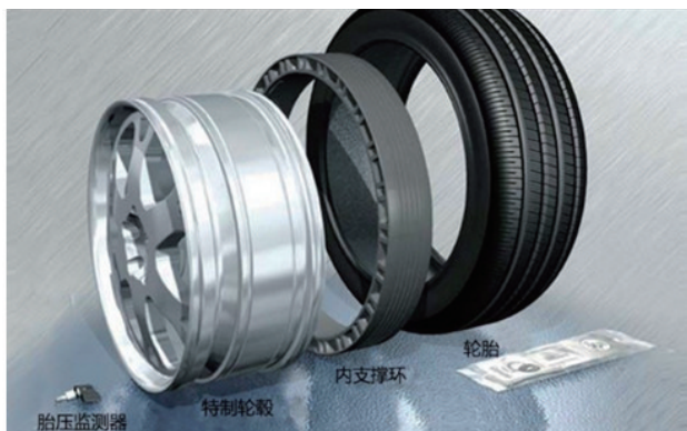
图10 米其林PAX系统的基本结构 Fig. 10 The basic structure of PAX system from Michelin company
