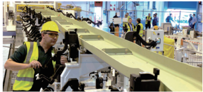
图9 Hot Drape Forming工艺成型的翼梁 Fig. 9 Composites wing spar manufactured by Hot Drape Forming
