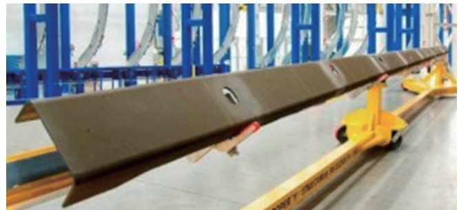
图10 ASFM工艺成型的 A350 复合材料机翼前梁 Fig. 10 Composites wing front spar of A350 manufactured by ASFM
