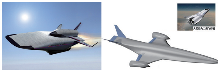
图 13 组合动力两级入轨重复使用运载器示意 Fig. 13 Schematic diagram of combined power two stage to orbit reusable launch vehicle
