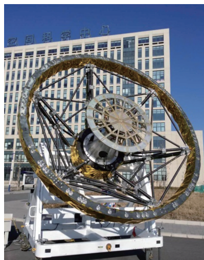
图1 中欧静止轨道毫米波大气探测仪样机 Fig.1 CAS-ESA geostationary millimeter wave atmospheric sounder prototype
