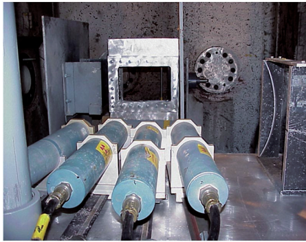
图2 第一阶段替代材料为玻璃/铅玻璃的气溶胶测试装置 Fig. 2 Aerosols testing device with glass/leaded glass in the first phase
