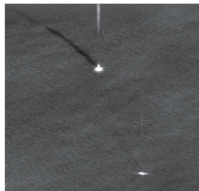
图2 C波段VV极化机载SAR获取的溢油图像 Fig. 2 Oil pictures captured by C-band VV-polarization airborne SAR
