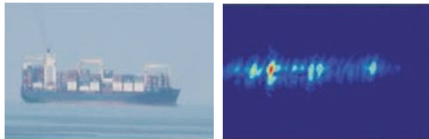
图9 微波光子雷达ISAR舰船目标高分辨成像示意 Fig. 9 ISAR ship image of microwave photonic radar
