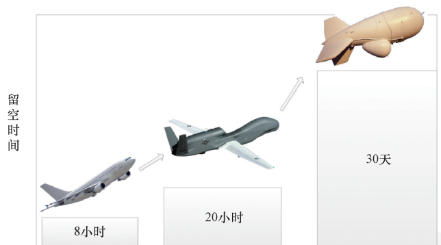
图5 系留气球与固定翼飞机的滞空时间对比 Fig. 5 Comparison of flying times of tethered aerostats and fixed-wing aircraft
