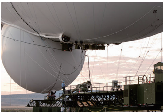
图 16 气球腹部防风罩内安装的是球载雷达系统 Fig. 16 Airborne radar system in the wind-shelter under the aerostat
