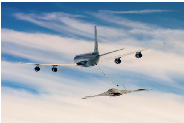
图3 X-47B无人机与K-707加油机进行自主空中受油试飞 Fig. 3 X-47B UCAV is making automatic aerial refueling trial with the K-707 tanker aircraft
