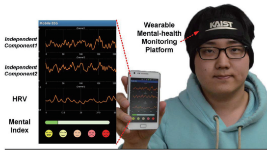
图9 精神状态监测可穿戴系统演示 Fig. 9 Demonstration of wearable mental state monitoring system
