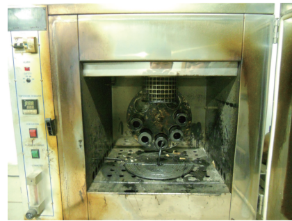
图2 沥青旋转薄膜加热试验 Fig. 2 Asphalt rolling thin film oven test
