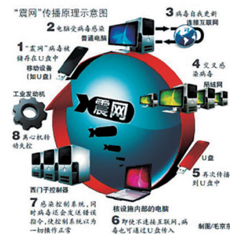
图4 “震网”病毒攻击核设施原理示意
