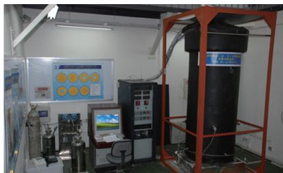
图 8 中国首台缓冲回填材料大型实验台架 Fig. 8 The first large-scale Mock-up facility for buffer and backfill material research in China
