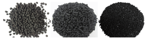
图3 球形碳(左)、柱状碳(中)、无定形碳形貌(右) Fig. 3 The morphology of formed spherical (left), columnar (middle) and irregular activated carbon (right)
