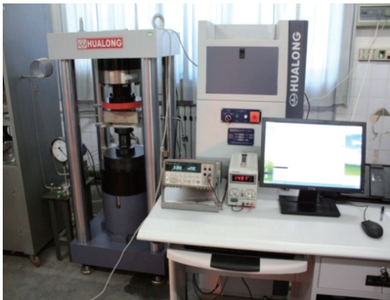
图1 LD-1A导流能力测试仪 Fig. 1 LD-1A conductivity meter
