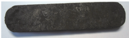
图3 煤岩样品实物 Fig. 3 Finished product of coal samples
