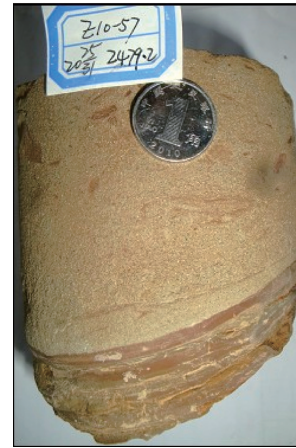
图3 港中油田中10-57井泥岩夹层—低缓倾角(滨I5) Fig. 3 Mud interbed from the well Zhong 10-57 in Gangzhong oilfield—the gentle dip angle
