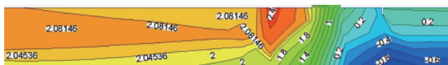
图 10 火源附近流速场稳态分布 (m/s) Fig. 10 Velocity field steady distribution near the fire (m/s)
