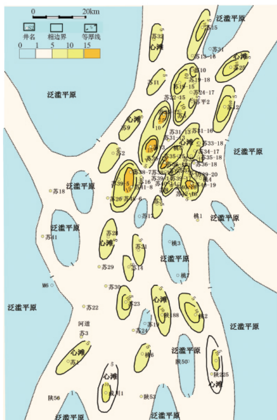
图3 苏里格气田盒8砂层厚度与沉积相图 Fig. 3 Thickness and sedimentary facies for under He 8 in Su Lige gas field
