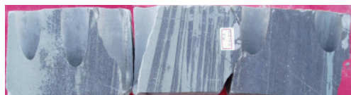
(a) 中 13 井 5131.54m, 含沥青灰色细砂岩, 发育低角度冲洗层理 (a) Development of low angle washing bedding with grey bitumen fine sandstone at 5131.54m of Well Zhong13
