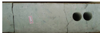
(f) 中 11 井 5003.5m, 块状粉砂岩可见生物扰动 (f) Blocky siltstone with visible bioturbation at 5003.5m of Well Zhong 11
