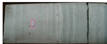
(b) 中 11 井 5014.4m, 灰色细砂岩, 发育流水波纹层理 (b) Development of water ripple bedding with grey fine sandstone at 5014.4m of Well Zhong11
