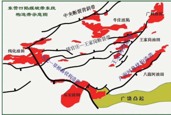
图1 东营凹陷缓坡带东段构造带示意 Fig. 1 Scheme of the tectonic zone at gentle slope belt in Dongying Sag
