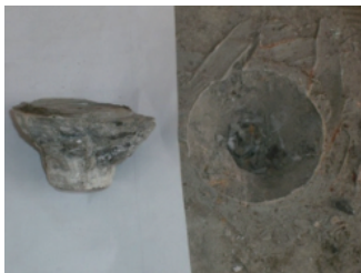
图5 有机植筋胶拔出效果 Fig. 5 Effect of pull-out by using organic anchorage
