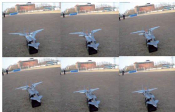
图 12 飞行器 F-15m 变翼过程示意 Fig. 12 Folding process of F-15m aircraft
