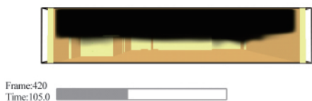
图 10 105s 时烟气蔓延状况 Fig. 10 Flue gas spreading conditions at 105s
