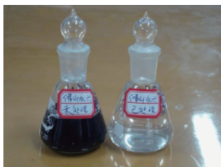
图 7 处理前(左)、后(右)水样对比照片 Fig. 7 Waster water before (left) and after (right) superconducting magnetic separation
