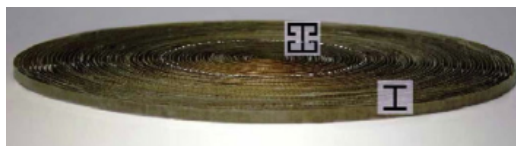
图 8 超材料制成的全方位电磁减震器 Fig. 8 Omnidirectional electromagnetic absorber made of metamaterials
