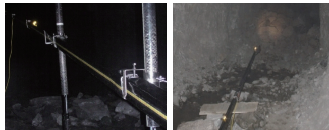
(a) 以碳化玻璃钢支架 (a) Supported by carbonization FRP bracket (b) 以石头和木板为支撑 (b) Supported by stone and wood
