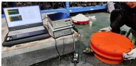
图7 实验用GIS腔体及盆式绝缘子 Fig.7 The GIS chamber and basin insulator for experiment
