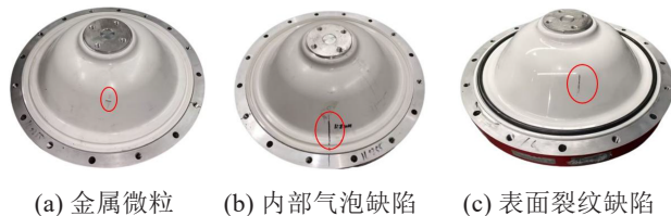
图8 实验用缺陷盆式绝缘子 Fig.8 Defect basin insulator for experimental
