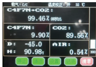
图6 C_4F_7N/CO_2 混合气体的混合比和微水检测结果 Fig.6 Mixing ratio and micro-water test results of C_4F_7N/CO_2 mixed gas
