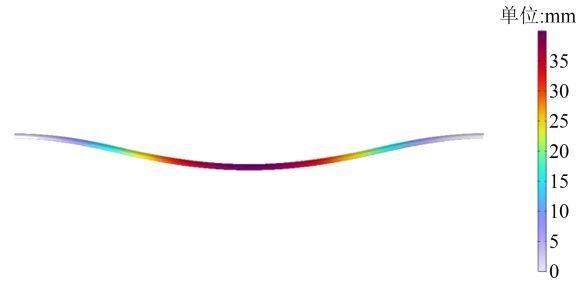
图5 垂直蛇形敷设电缆的位移分布情况 Fig.5 Displacement distribution of cable under vertical serpentine laying
