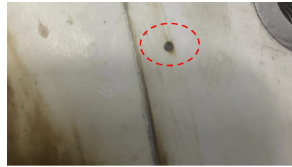
图3 表面浅层异物放电现象 Fig.3 Discharge phenomenon of shallow inclusions on the surface
