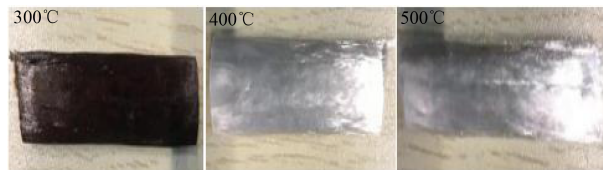
图15 不同温度下热老化芯棒的外观形貌 Fig.15 Appearance of mandrel thermal ageing at different temperatures
