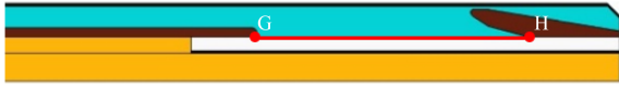
图6 10 kV 电缆接头中的仿真路径 Fig.6 Simulation path in 10 kV cable joint
