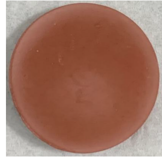
图4 样品表面出现二次粉化现象 Fig.4 Secondary pulverization phenomenon occurred on the surface of sample
