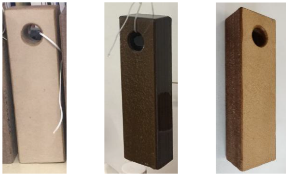
(a)浸油前 (b)浸油后露空10天 (c)浸油后露空2个月 图1 绝缘件露空试验
