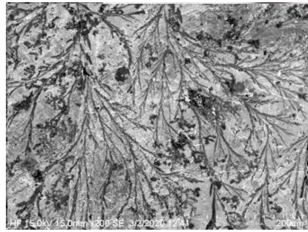
图1 通电不良接触器触点元件表面SEM图 Fig.1 SEM image of contact element surface for poorly energized contactor
