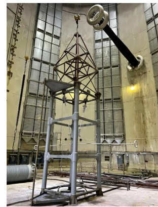
(c)污秽闪络试验样品布置
