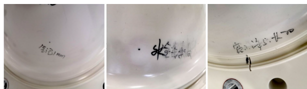
(a)气泡缺陷 (b)杂质缺陷 (c)裂纹缺陷
