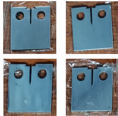
(a) CT 试样实物 (a) Physical CT specimen
